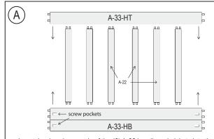
Insert the dowels on ends of the (6) A-22 headboard pickets into the corresponding holes in the A-33-HT and A-33-HB as pictured. Be sure the screw pockets of the A-33-HB headboard bottom are facing you and that the screw pockets of the A-33-HT headboard top are NOT facing you.
